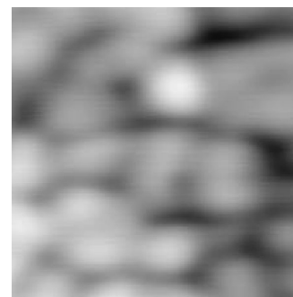
Figure 1. A NC-AFM image of PZT layer sample under X-ray irradiation, 70 × 70 nm 2 , Δ f = -20 Hz, A 0 = 27 nm.
