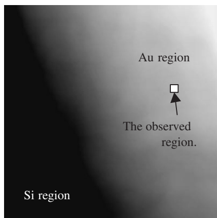
Figure 2. NC-AFM image of partial Au-deposited Si surface, 3.5 \times 3.5 \mu\text{m}^2 , \Delta f = -20 \text{ Hz} , A_0 = 27 \text{ nm} .
